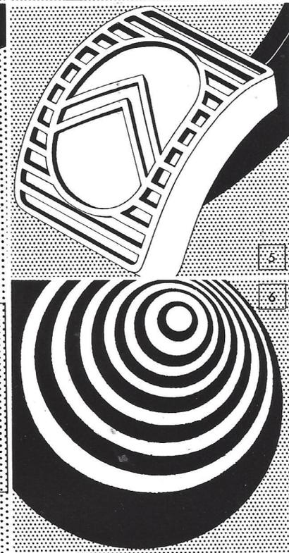
1) This is a disc brake. But it is no ordinary one: it is a Citroën disc brake which is fitted to the ID and DS front wheels (where the load is greatest). Disc brakes are better cooled and do not fade or ovalize. In 1955, Citroën was the first to fit disc brakes as standard equipment on production cars.
